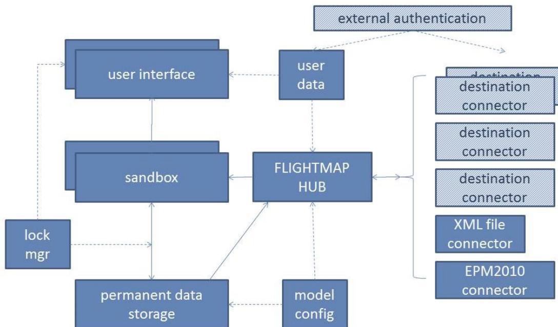
**Figure 1 FLIGHTMAP Connectivity Architecture (shaded components require custom development).**
